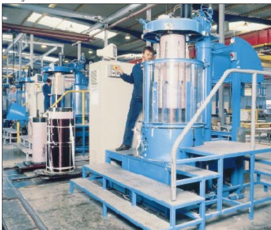
winding an HV coil
