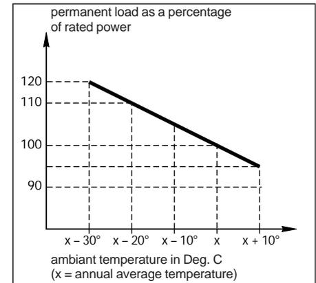
one can operate a transformer designed for operation in ambient of 40 Deg.C at higher temperatures by reducing the rating as shown in the table.
