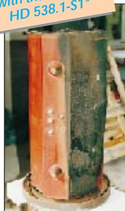
Trihal transformer coil after the test F1.
