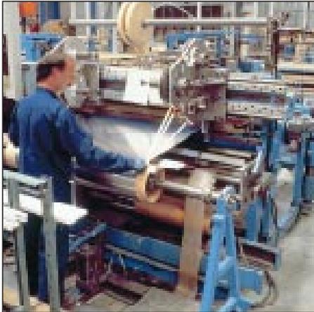
winding an HV coil
