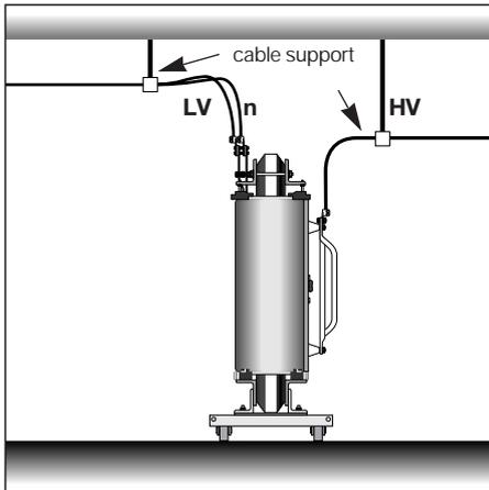
figure 2 - standard HV and LV connections from below
