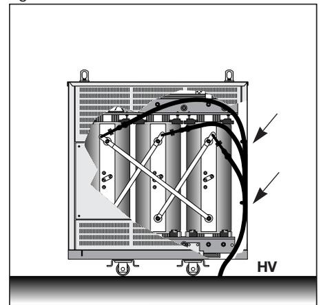
figure 3 - HV connections with plug in connectors (option)
