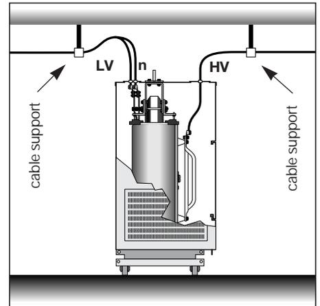
figure 2 - standard HV connection from below
