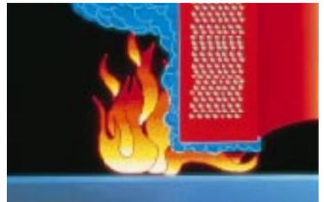
2<sup>nd</sup> anti-fire effect : barrier of water vapour.
