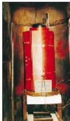
test F1 on a complete Trihal transformer coil.
