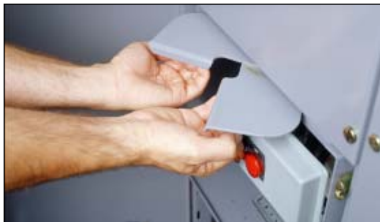
Figure 48: Pulling the Twin Handles of the Cam Mechanism Forward
