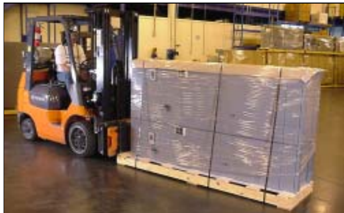
Figure 3: Moving an MCC with a Fork Truck
