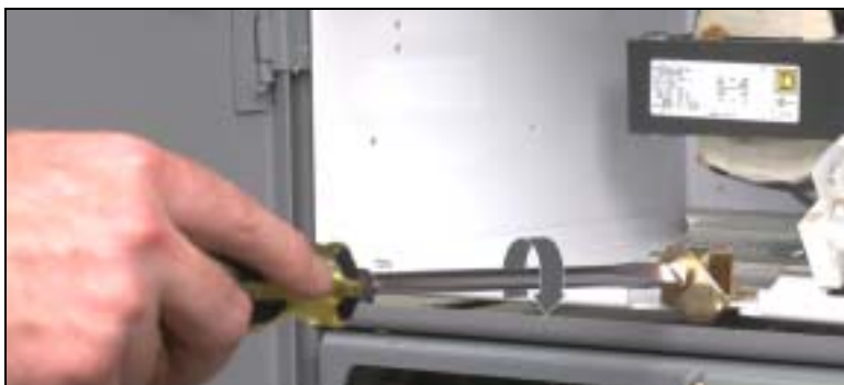
Figure 50: Tightening the Control Unit Lock-In Panel (when supplied)
