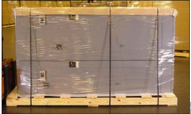
Figure 2: Packaged Export Motor Control Center
